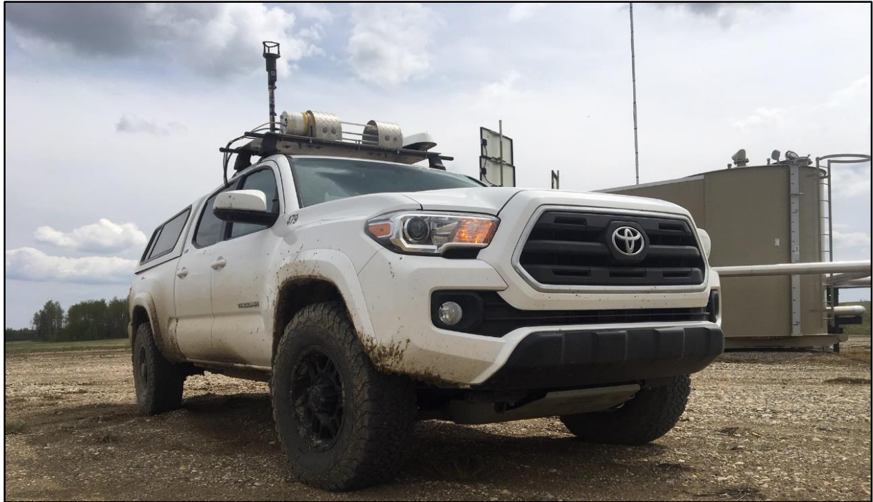
Figure 2: The PoMELO system mounted on the roof of a standard field truck.
