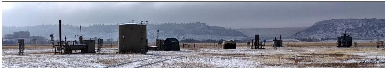
Figure 1: Mock equipment at the METEC site. The facility uses real production equipment that has been modified to have hidden leak points throughout. Participants cannot tell where emissions are located – making the facility a globally-leading test platform for upstream oil and gas LDAR technologies.
